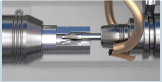
Internal cylindrical grinding
