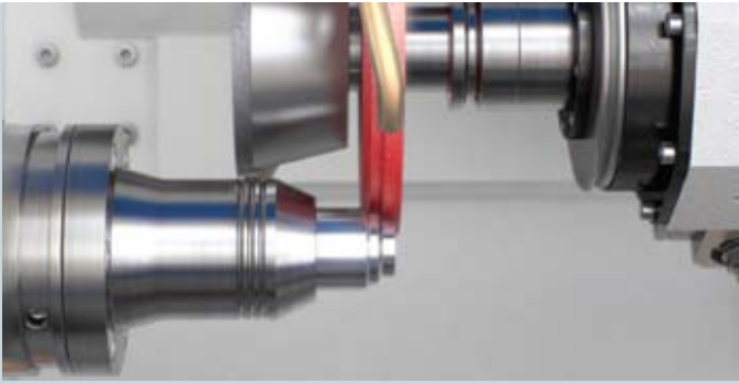
External cylindrical grinding
