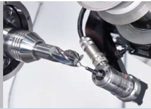
Swivelling probe for position determination and measurement of the workpieces
