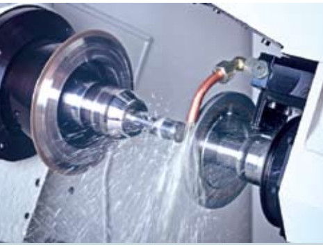
Dressing with drive from the workpiece axis
