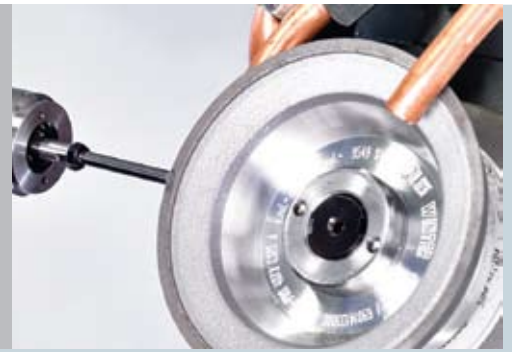
Additional probe for measuring the grinding wheels in the machine
