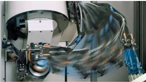
Swivellable gripper for pallet or chain magazine
