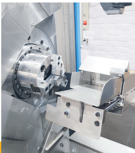
Parts discharge via a chute
