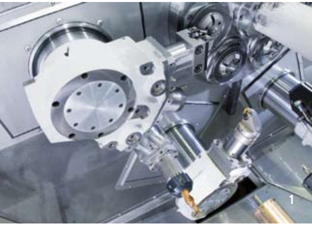
Fig. 1, Image sequence at top, from left to right: Free configuration of the tool heads in all spindle positions.
